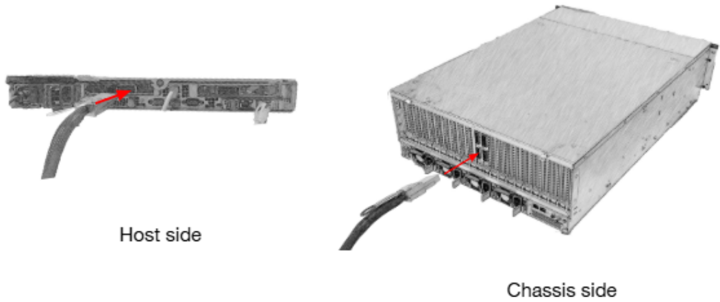
Figure 49. Host and Chassis Connections Using CDFP Cables
