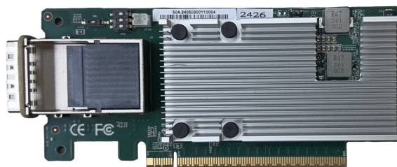
Figure 17. C01 Host Adapter Card – Top View
