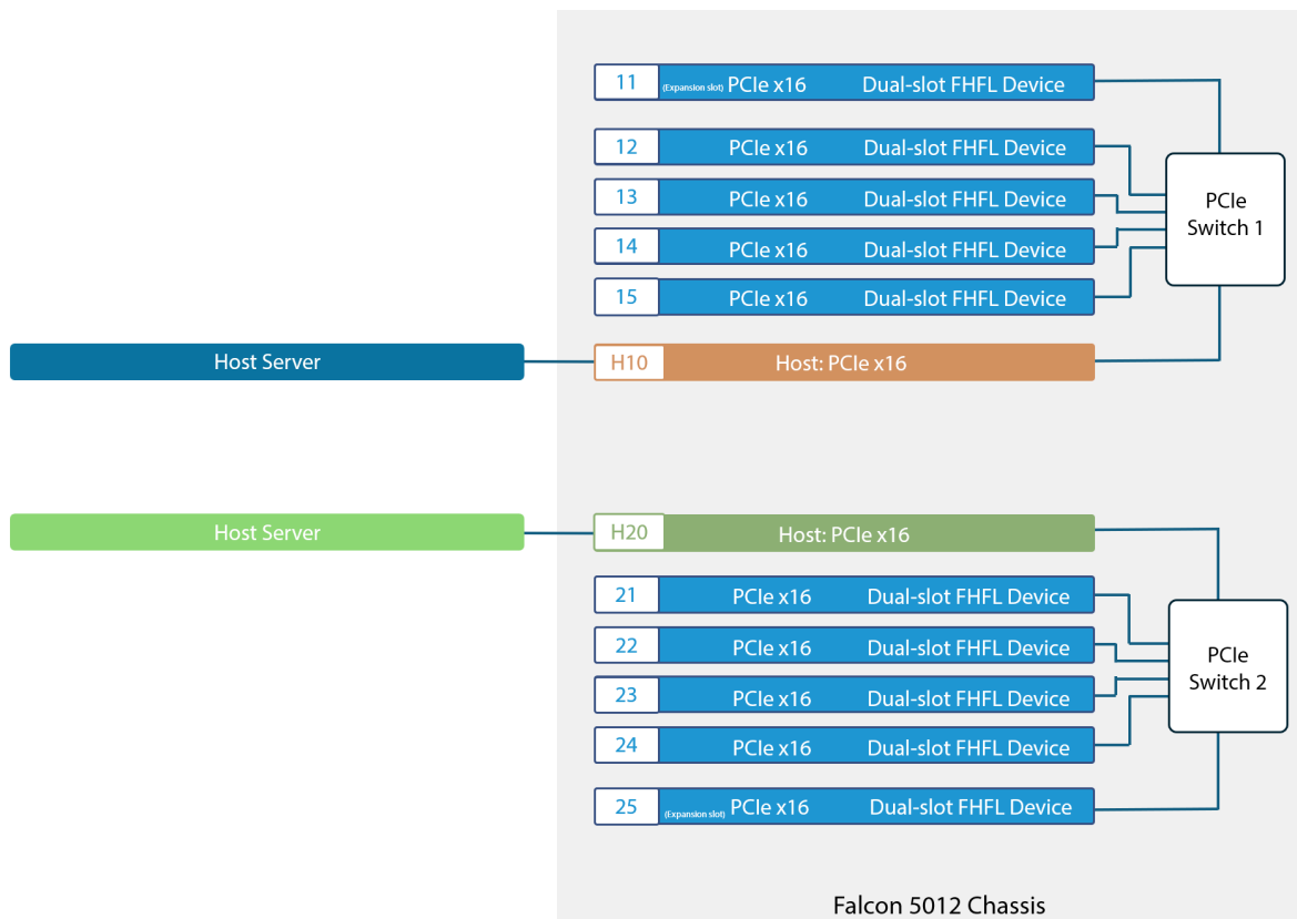
Figure 9. Block diagram of Standard Mode architecture topology with 2 x16 hosts and 10 GPUs
