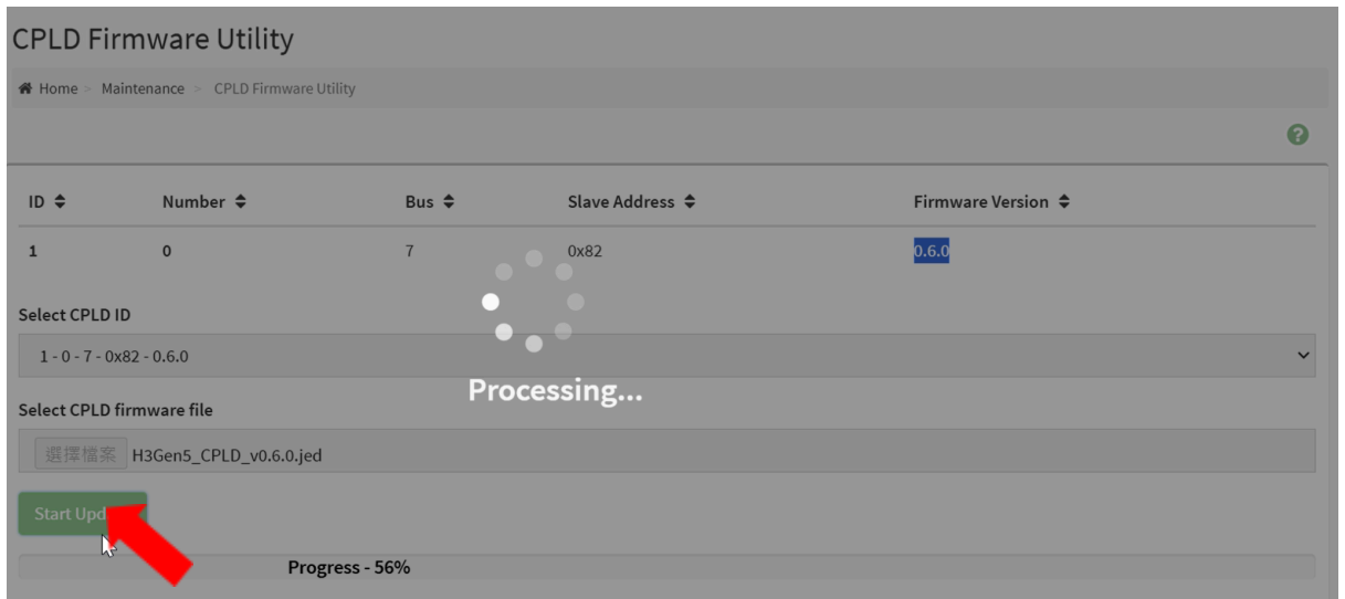
Figure 107. Processing During CPLD Firmware Update
