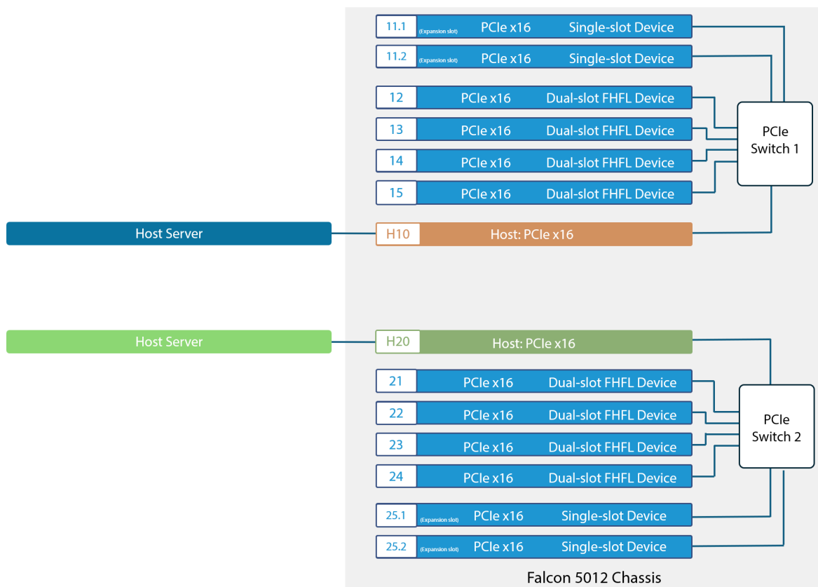
Figure 12. Block diagram of Standard Mode architecture topology with 2 x16 hosts and 8 GPUs + 4 NICs
