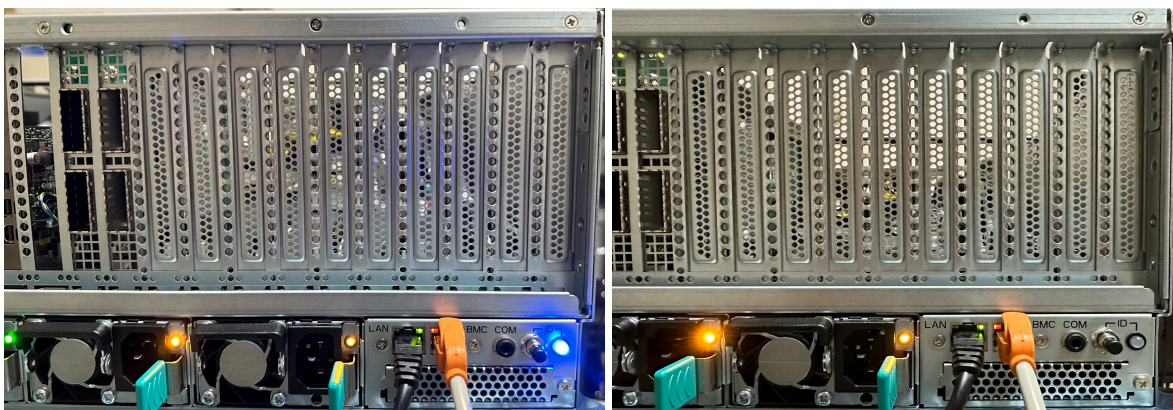
Figure 25. UID Light Blinks Twice Before System Power-On
