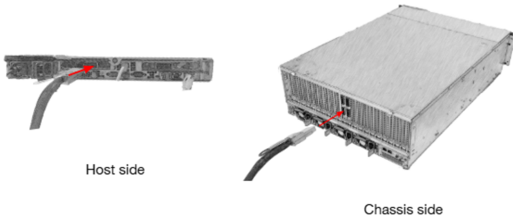
Figure 75. Host and Chassis Connections Using CDFP Cables
