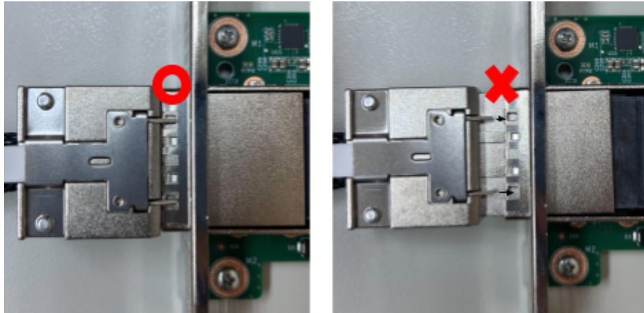
Figure 39. Picture of properly connecting the CDFP cable with the CDFP connector
