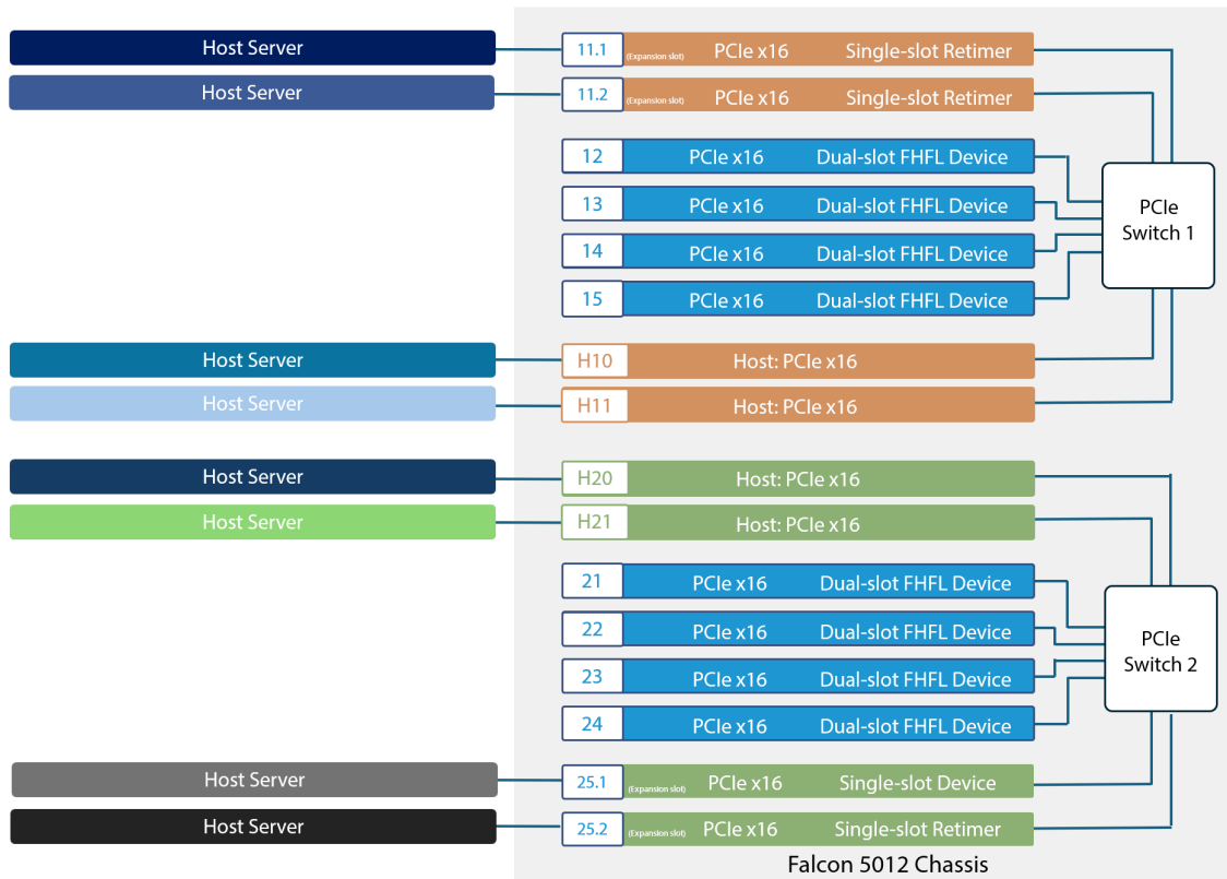
Figure 15. Block diagram of Advanced Mode architecture topology with 8 x16 hosts and 8 GPUs
