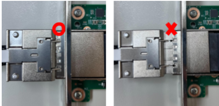
Figure 123. Picture of properly connecting the CDFP cable with the CDFP connector
